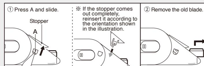
① While pressing part A with a thinly-pointed object, slide the stopper in the direction of the arrow.
